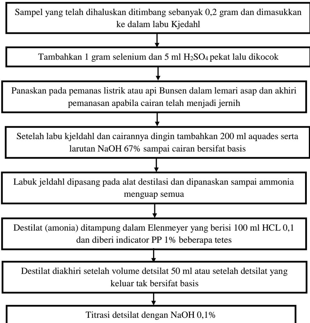
**Gambar 3.3** Diagram Alir Proses metode Kjeldahl
