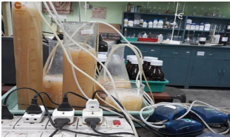
**Fig. 1** Experimental setup of suspended growth batch reactor
